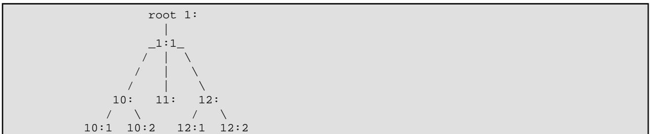
When enqueueing a packet, at each branch the filter chain is consulted for a relevant instruction. A typical setup might be to have a filter in 1:1 that directs a packet to 12: and a filter on 12: that sends the packet to 12:2.
