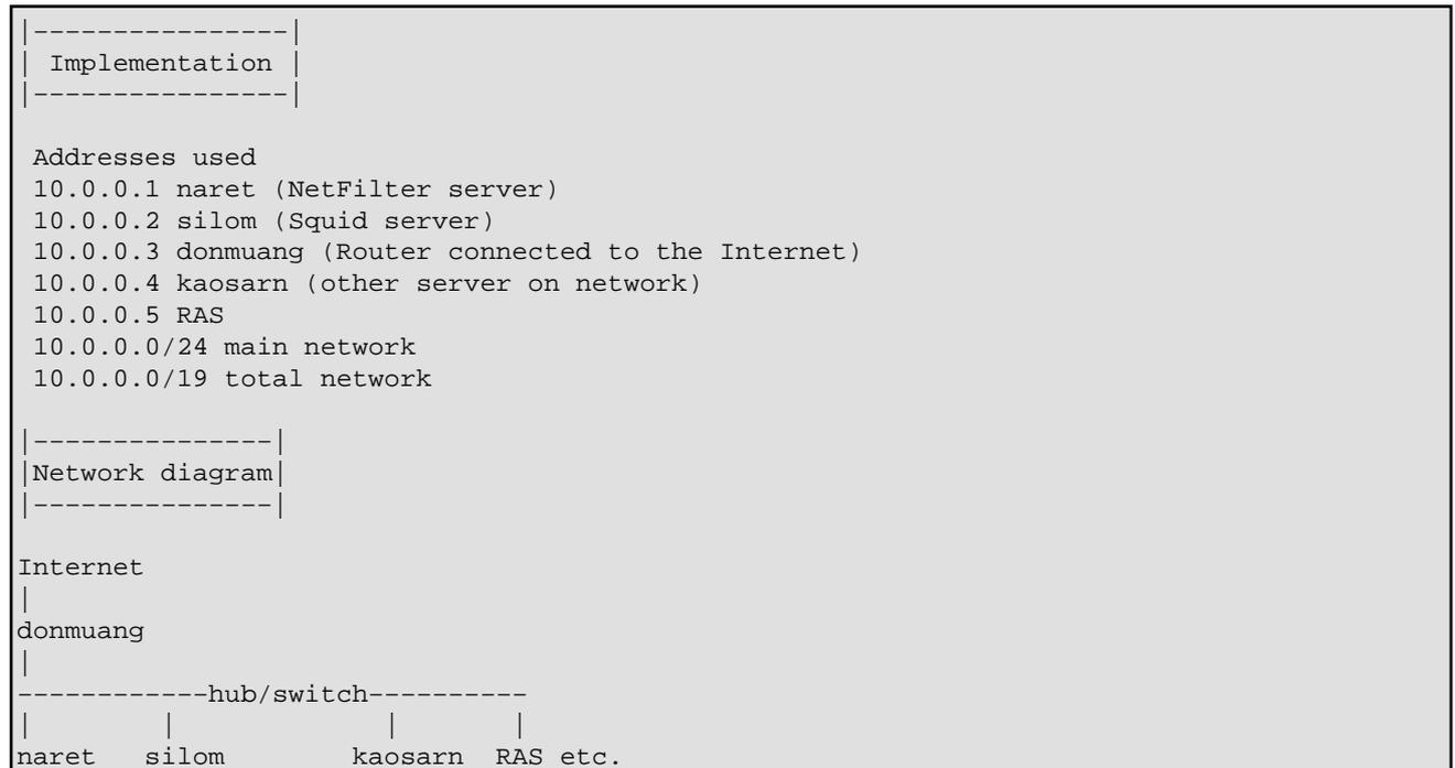
First, make all traffic pass through naret by making sure it is the default gateway except for silom. Silom's default gateway has to be donmuang (10.0.0.3) or this would create web traffic loop.
