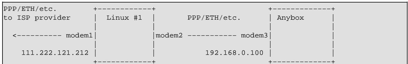
In the above drawing, a Linux box with IP\_MASQUERADING is installed as Linux #1 and is connected to the Internet via PPP, Ethernet, etc. It has an assigned public IP address of 111.222.121.212. It also has another network interface (e.g. modem2) connected to allow incoming network traffic be it from a PPP connection, Ethernet connection, etc.
