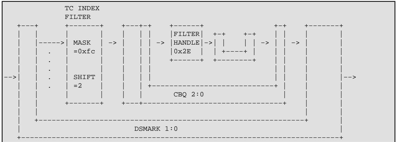
The packet arrives, then, set with 0xb8 value at DS field. As we explained before, dsmark qdisc identified by 1:0 id in the example, retrieves DS field and store it in `skb->tc_index` variable. Next step in the example will correspond to the filter associated to this qdisc (second line in the example). This will perform next operations:
