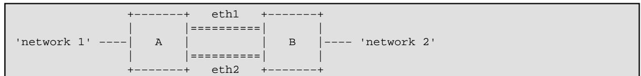
A and B are routers, and for the moment we'll assume both run Linux. If traffic is going from network 1 to network 2, router A needs to distribute the packets over both links to B. Router B needs to be configured to accept this. Same goes the other way around, when packets go from network 2 to network 1, router B needs to send the packets over both eth1 and eth2.
