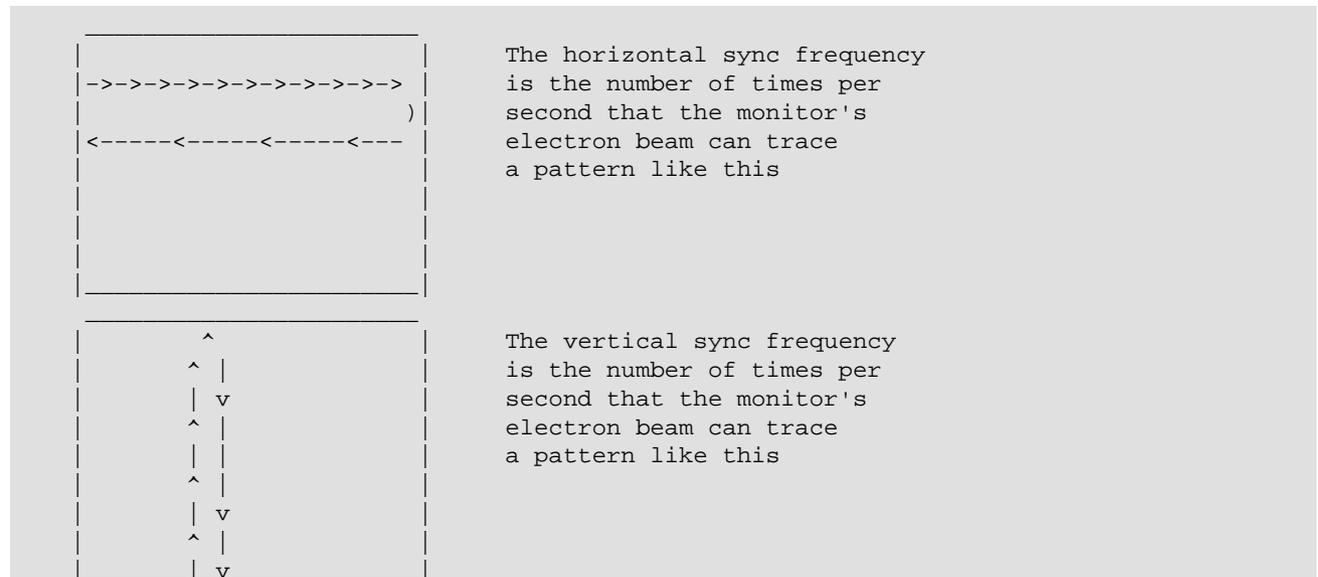
Remember that the actual raster scan is a very tight zigzag pattern; that is, the beam moves left-right and at the same time up-down.
