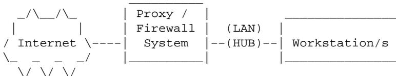
You can put the proxy server on your LAN as will. In this case the firewall should have rules to only allow the proxy server to connect to the Internet for the services it is providing. This way the users can get to the Internet only through the proxy.
