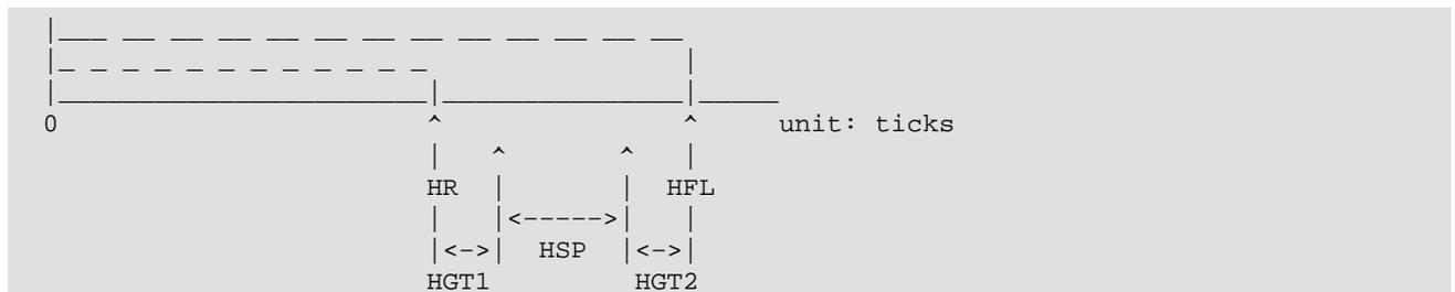
Now, we would like to place a sync pulse of length HSP as shown above, ie, between the end of clock ticks for display data and the end of clock ticks for the entire frame. Why so? because if we can achieve this, then your screen image won't shift to the right or to the left. It will be where it supposed to be on the screen, covering squarely the monitor's viewable area.
