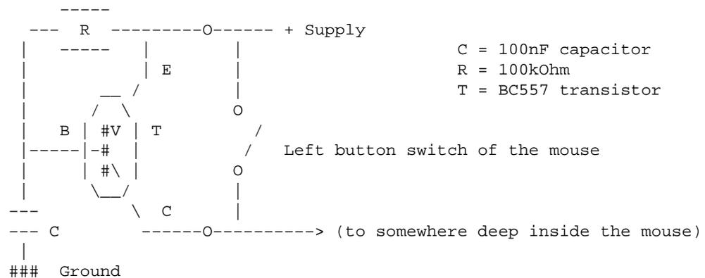
The test mouse was a no-name model MUS2S – whether this works in other mice depends on the circuit of the mouse; if the switch is connected to ground and not to +Supply, an npn-transistor like the BC547 should work; R and C have to be swapped then, too.
