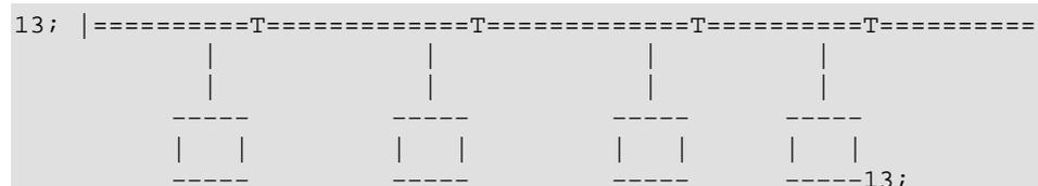
where the `|' at either end represents a terminator, the `=====' represents a length of coaxial cable with BNC plugs at either end and the `T' represents a `T piece' connector. You should keep the length of cable between the `T piece' and the actual ethernet card in the PC as short as possible, ideally the `T piece' will be plugged directly into the ethernet card.
