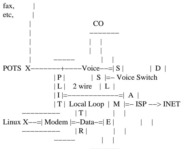
Figure 2: DSL Splitterless (a.k.a. filtered) Block Diagram
