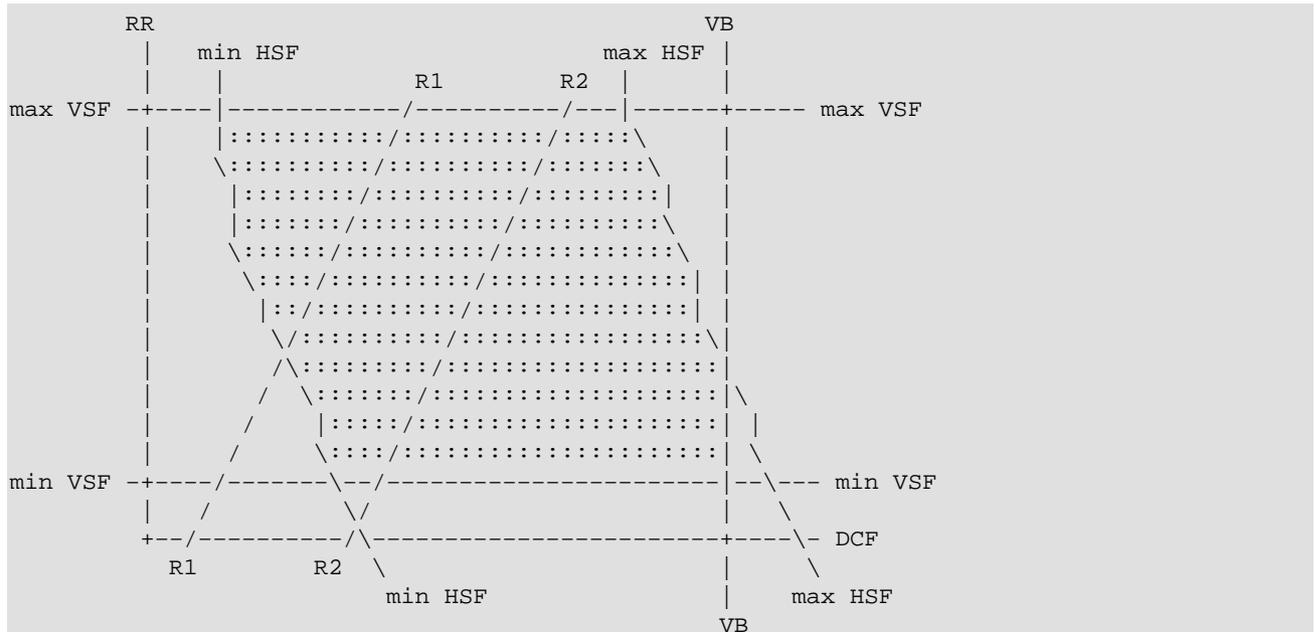
This is a generic monitor mode diagram. The x axis of the diagram shows the clock rate (DCF), the y axis represents the refresh rate (RR). The filled region of the diagram describes the monitor's capabilities: every point within this region is a possible video mode.
