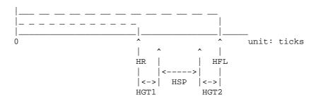
Now, we would like to place a sync pulse of length HSP as shown above, ie, between the end of clock ticks for display data and the end of clock ticks for the entire frame. Why so? because if we can achieve this, then your screen image won't shift to the right or to the left. It will be where it supposed to be on the screen, covering squarely the monitor's viewable area.
