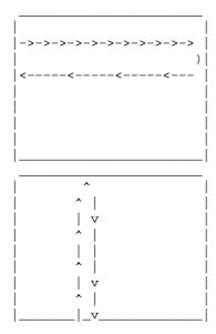
The horizontal sync frequency is the number of times per second that the monitor's electron beam can trace a pattern like this
