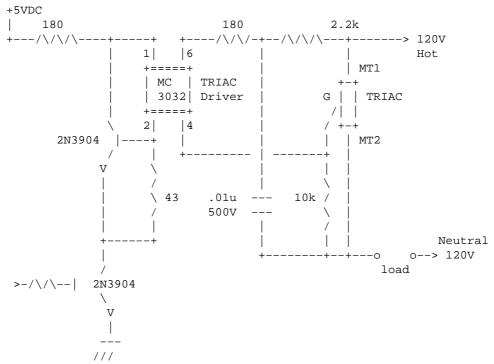
You should change resistors accordingly for 220V.
