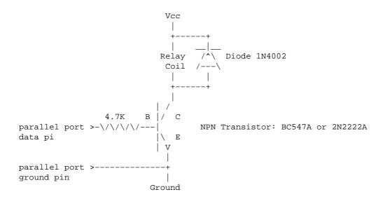
Connect Vcc with the same voltage as the relay type (usually 5 or 12V). Obviously, the relay's specifications should be reasonable for your coffee—machine.
