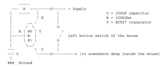
The test mouse was a no-name model MUS2S – whether this works in other mice depends on the circuit of the mouse; if the switch is connected to ground and not to +Supply, an npn-transistor like the BC547 should work; R and C have to be swapped then, too.
